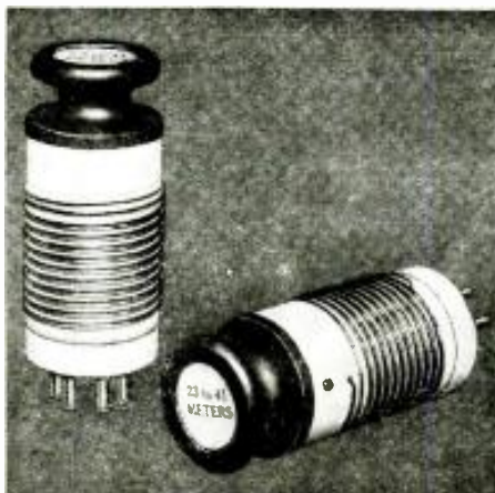
Improved plug-in coils of the 6-pin type, the wire being wound on grooved isolantite forms. The wavelength rating appears in a protected label set into the knob.
